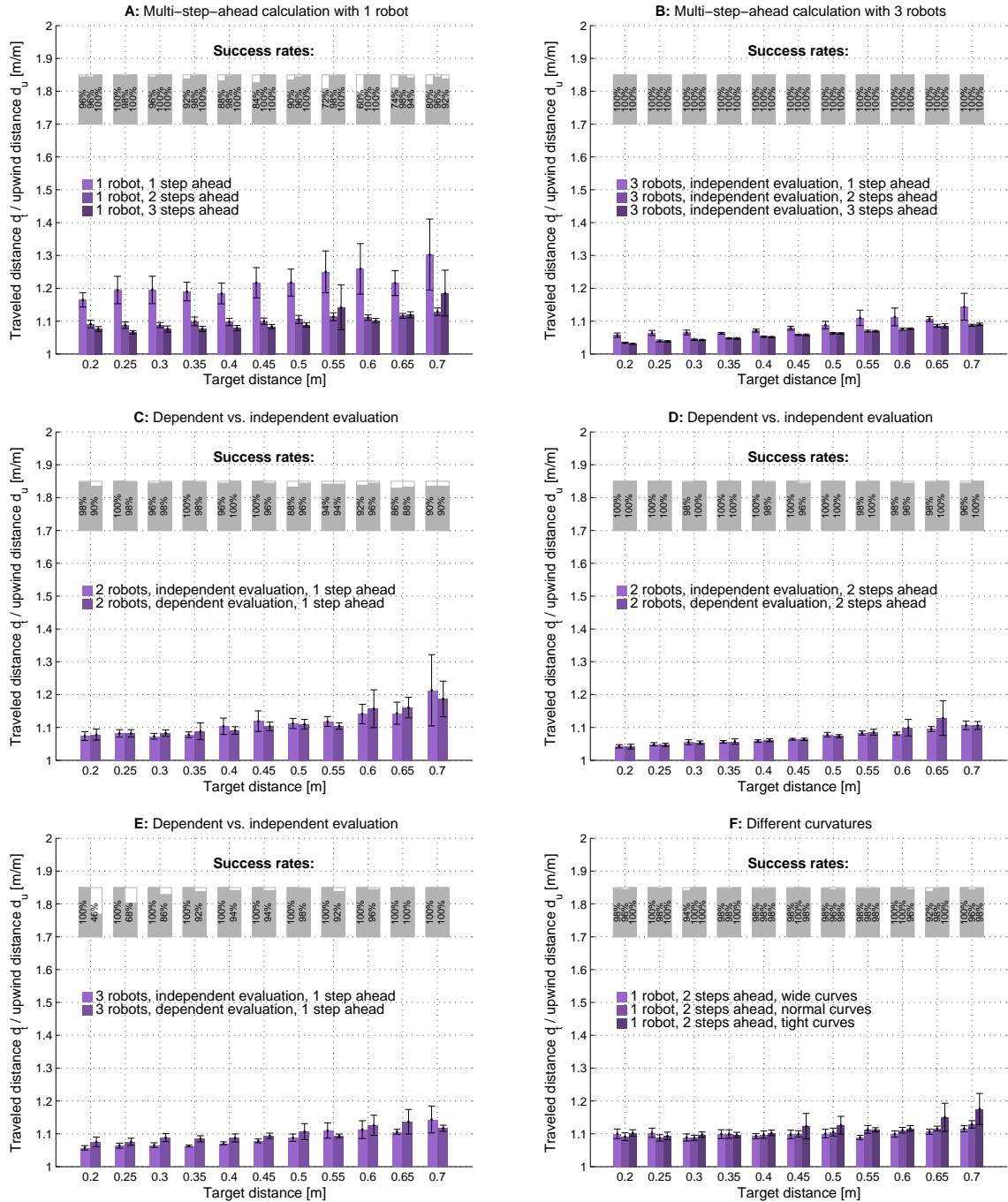
Figure 4.9: Results obtained with the point simulation assuming absolute localization. A, B: Influence of multi-step-ahead evaluation with 1 robot resp. 3 robots. C, D, E: Dependent vs. independent evaluation with 2 robots with 1-step-ahead evaluation, 2 robots with 3-step-ahead evaluation, and 3 robots with 1-step-ahead evaluation. F: Effect of the curvature parameter.
